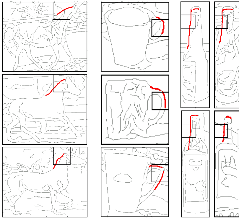
Fig. 5. One of the most important window descriptor dimensions, according to SVM training ( k = 2 ). Each column shows a few training images for a class, along with one of the ‘ k AS type + tile’ combinations which are given the highest weight by the SVM.
